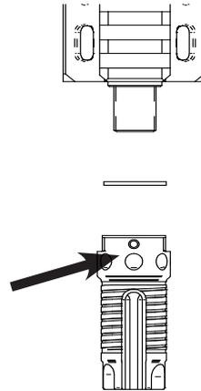
**2 Re-attach the muzzle device and torque to 15-20 ft-lbs and ensure the alignment pin is in-line with the gas block to achieve the 12 o'clock position, +/- 3 degrees.**
