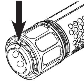
**4 Pull the suppressor back onto the muzzle device so the alignment notch and the alignment pin achieve the 12 o'clock position.**
