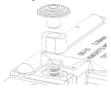
5. Continue tightening button until it sits flush with receiver while pushed. Magazine release lug should clear inside edge of magazine well and magazine should fall free.
