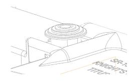
6. Install & tighten set screw (3/32" Hex). (Medium strength Loctite on Set Screw recommended.)
