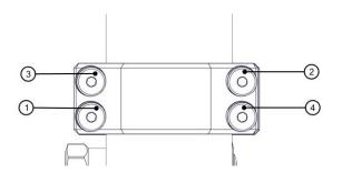
1. Install scope mount to receiver rail finger tight.
