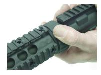
3. Torque FF RAS Barrel Nut to 31ft. lbs. or greater if necessary for gas tube clearance. Do not exceed 80 ft. lbs.
