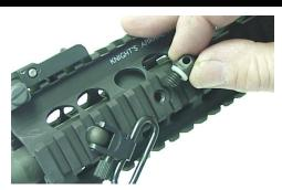
9. Standing Front Sight may be modified as shown above for assembly to the long FF RAS, or use of a KAC Low Profile Gas Block (PN: 99204) as shown on barrel.
