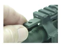
4. Insert two for 5.56; (or three for 7.62), Barrel Nut Pins, one at 9 & one at 3, and/or 6 o'clock for 7.62.
