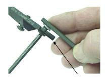
NOTE: If the Low Profile PEQ-2 Mount is to be used with Nut Plate, pre-assemble spacers to the shank of the mounts rear screw.
