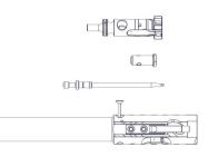
1. Wipe Bolt Carrier and Bolt Components clean and Dry.
