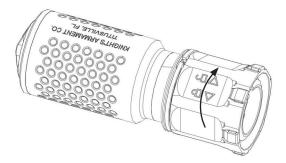
3. Firmly hand tighten the locking collar by turning the locking collar counterclockwise (to the left).
